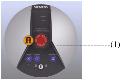
Prisma (control room quench buttons are the buttons labeled (1))
